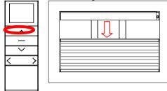
\* When the middle rail reach the bottom, the bottom rail & middle rail will go up together.
