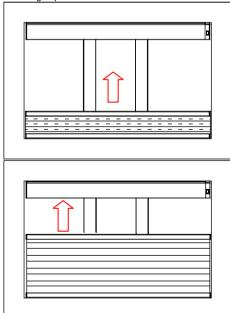
\* When middle rail meet the head rail, it is drop limit.
